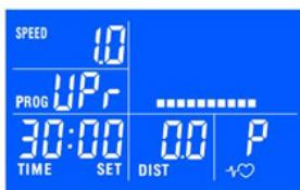
Use ^/v buttons to program speed and incline for each segment, press ENTER to confirm.
