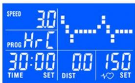
Use ^/v buttons to program target heart rate, press ENTER to confirm.
