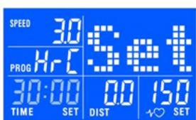
Press START: the treadmill will run at 3 km/h for 2 minutes as warm-up: adjust elevation manually.
